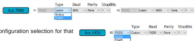
All serial ports support Modbus RTU protocol. The PLCs are slave devices. The default device address is 1 but can be configured to any desired address via vBuilder.
